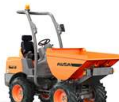
D120AHA 2,600 lb UNLOADING SYSTEM HIGH POWER 20.9 hp WIDTH 47.6 in TRANSMISSION HYDROSTATIC
