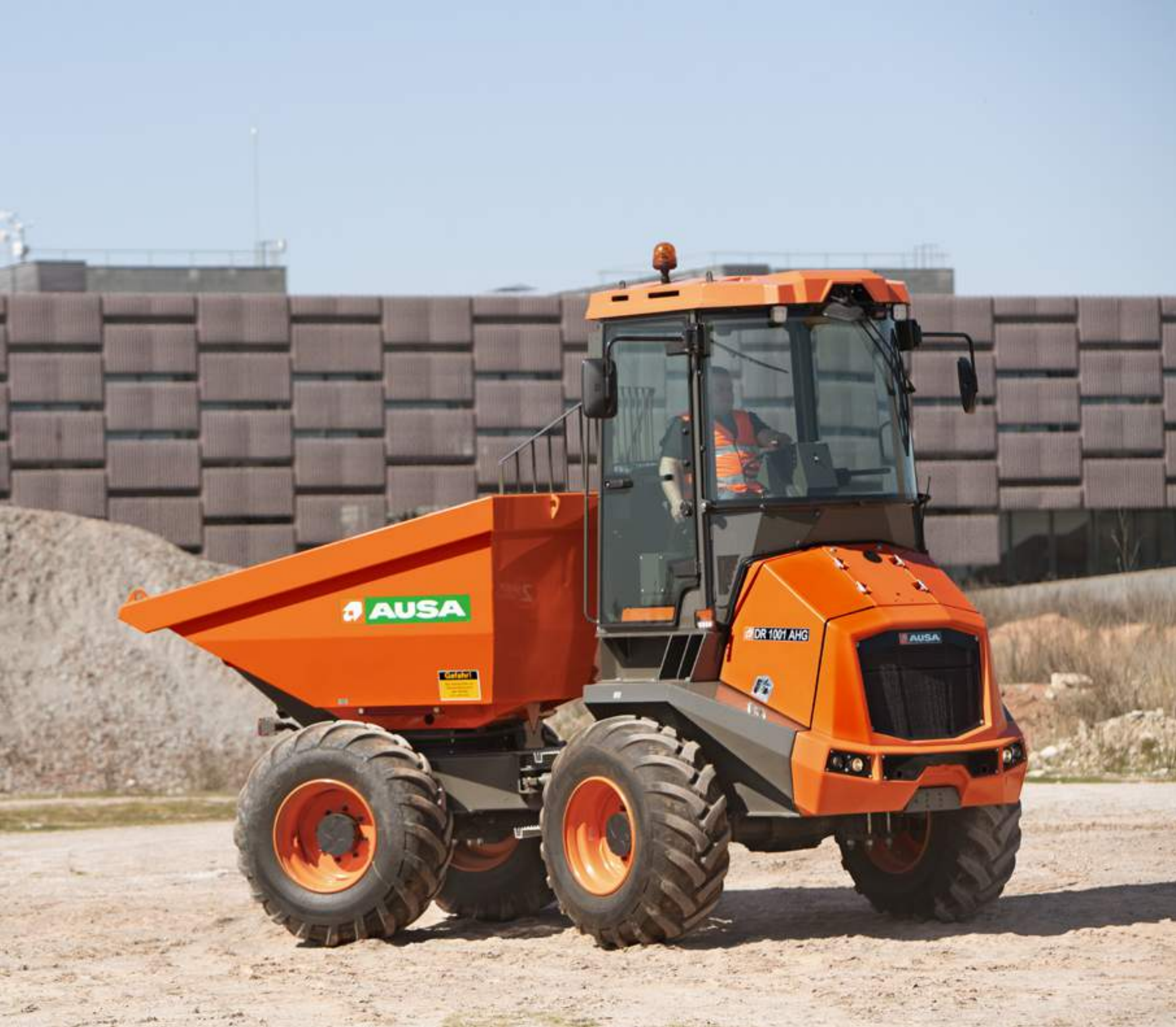
DR601AHG 13,200 lb UNLOADING SYSTEM ROTATING POWER 74.3 hp WIDTH 87 in TRANSMISSION HYDROSTATIC
