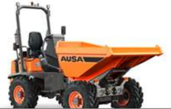
D301AHG 6,600 lb UNLOADING SYSTEM ROTATING POWER 24.8 hp WIDTH 68.9 in TRANSMISSION HYDROSTATIC
