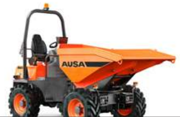
D450AHG 9,900 lb UNLOADING SYSTEM ROTATING POWER 44 hp WIDTH 73.6 in TRANSMISSION HYDROSTATIC
