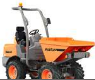
D120AHG 2,600 lb UNLOADING SYSTEM ROTATING POWER 20.9 hp WIDTH 47.6 in TRANSMISSION HYDROSTATIC
